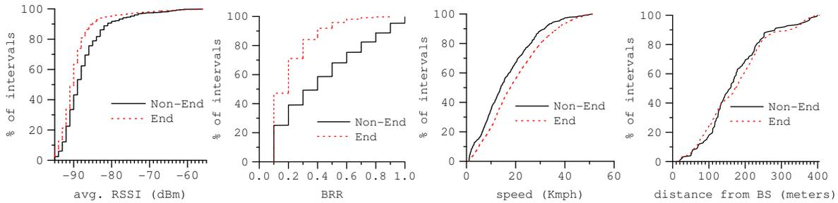
**Figure 6: Gray periods are hard to predict based on current measurements. The graphs plot the CDFs of four measures in 1-second intervals immediately preceding a gray period (“End”) and in other 1-second intervals (“Non-End”).**
