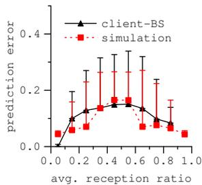
**Figure 11: Predicting performance at a location based on historical data is feasible. The graph plots the prediction error as a function of the average reception ratio observed in the previous day. The lines connect the mean and the whiskers depict the 90th percentile error.**
