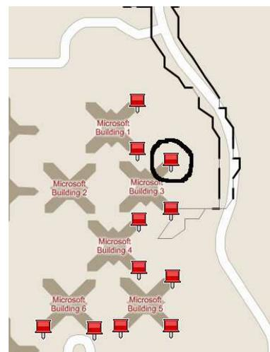
**Figure 3: Gray periods can occur even close to the BS. The figure shows the experience of the van in an example round with respect to the circled BS. Thick lines represent regions where beacons were received without a silent period of at least 2s. Thin lines represents the complement.**
