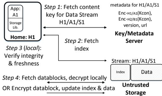
**Figure 3: Steps during reads and writes for application A1 in home H1 accessing stream H1/A1/S1.**
