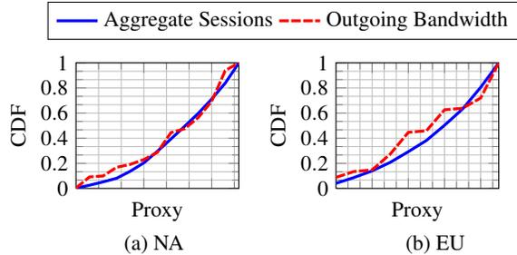
**Figure 9:** Distribution of bandwidth and sessions across proxies. User sessions are mapped to the closest proxy. Bandwidth per proxy is measured as aggregate bandwidth of all directly attached links.
