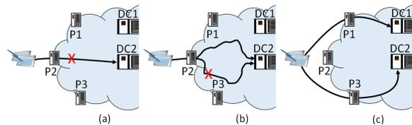
**Figure 2:** *Spatial modulation via joint coordination. (a) Path between P2 and DC2 is congested. (b) WAN TE alone cannot resolve this congestion because other paths between P2 and DC2 have low available capacity. (c) Congestion is resolved when user-to-proxy mapping and WAN TE are done jointly, moving users to other proxies with uncongested paths to DCs.*
