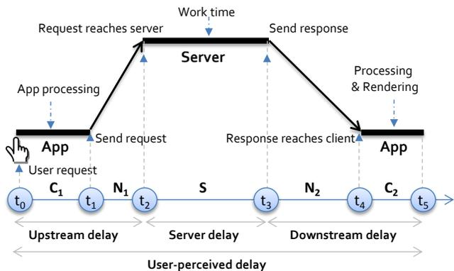
Figure 1: A typical transaction in an interactive app.
