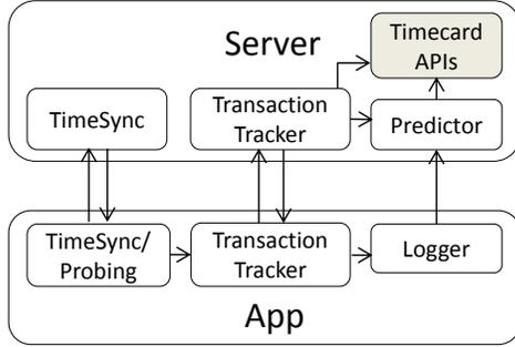
**Figure 2: Timecard Architecture.**
